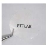
High transparency is maintained on the EVA thin film after adding the nano cellulose.
